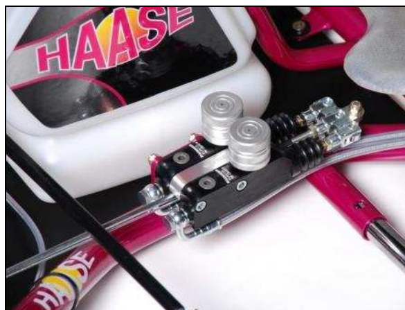
new double brake pump system
