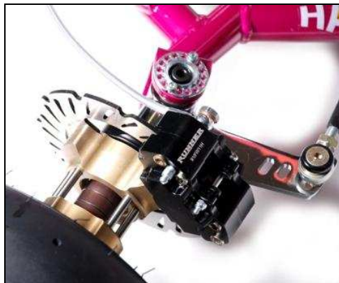
KF front brake and new caster camber pills
